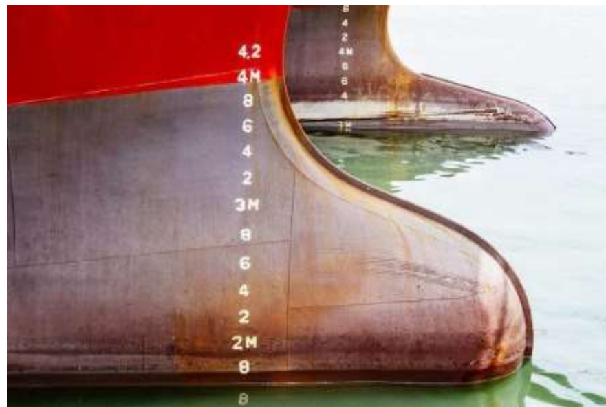
Figure 6 Draft of a cargo vessel
